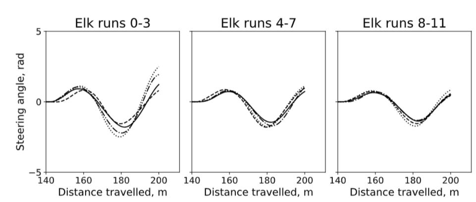
Cautious control on elk test maneuvers, with high  $\omega_{\sigma}$  (using BNN).
