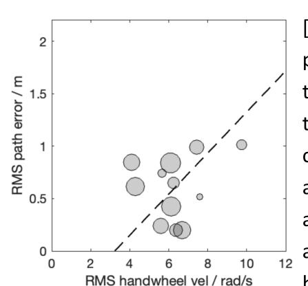
[1][3] Performance of human participant in experiment with repeated elk test maneuvers (see maneuver layout to left). Run number indicated by increasing marker size. Driver learning apparent as both metrics improve and behavior seen in run-to-run variability and trade-off in prioritisation between metrics. This participant
