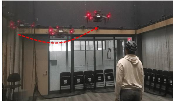
Fig. 1. Capturing images with a flying camera for the high-fidelity reconstruction of a dynamic actor. We build a drone system to capture a dynamic actor’s high-fidelity 3D reconstruction and study the view planning strategy for better reconstruction quality.
