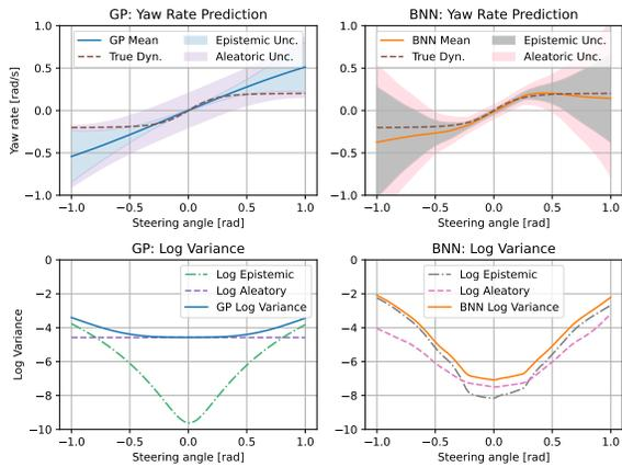
Fig. 1: GP and BNN internal model predictions for vehicle dynamics. In the top right figure uncertainties are stacked.
