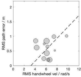
Fig. 3: Human results on elk test with adventurous driver [7], [4]. Maneuver number shown by increasing marker size.
