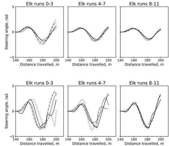
Fig. 5: Driver model steering traces with BNN internal model for repeated elk tests with high (top 3 plots) and low (bottom 3 plots) penalties on prediction variance to represent cautious and adventurous control respectively.
