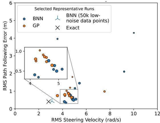
Fig. 4: Driver model elk test results with GP and BNN. The markers show statistically selected<sup>1</sup> representative maneuver series of 12 elk test runs from 100 repeats of this with each model. Maneuver number is indicated by marker size, with the first maneuver the smallest and the last (12<sup>th</sup> maneuver) the largest. The same vehicle/cost/noise parameters and dataset sizes are used for both models.
